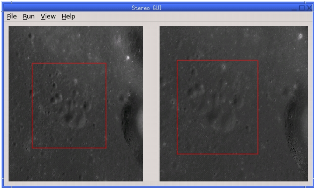
Fig. 13.3: An illustration of stereo_gui . The stereo command will be run on the regions selected by red rectangles.
