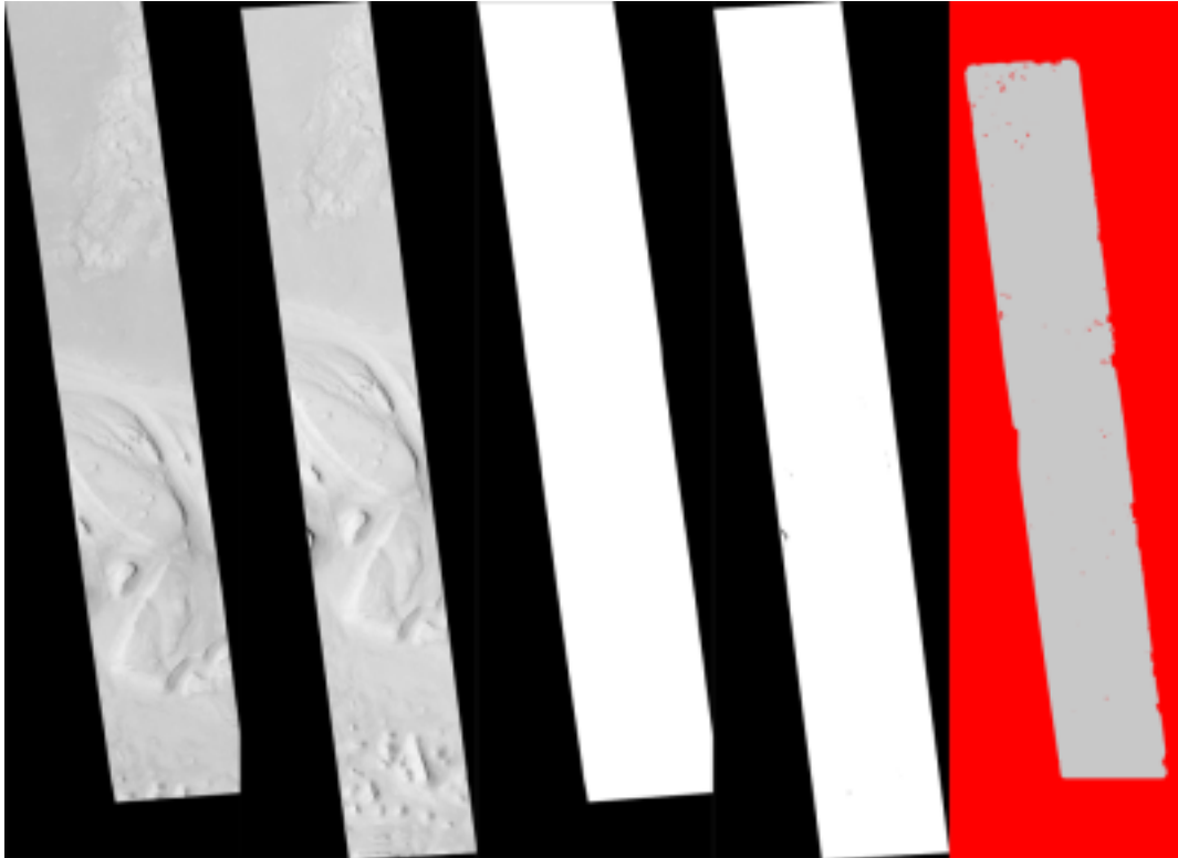
Fig. 5.1: These are the four viewable .tif files created by the stereo program. On the left are the two aligned, pre-processed images: ( results/output-L.tif and results/output-R.tif ). The next two are mask images ( results/output-lMask.tif and results/output-rMask.tif ), which indicate which pixels in the aligned images are good to use in stereo correlation. The image on the right is the “Good Pixel map”, ( results/output-GoodPixelMap.tif ), which indicates (in gray) which were successfully matched with the correlator, and (in red) those that were not matched.
